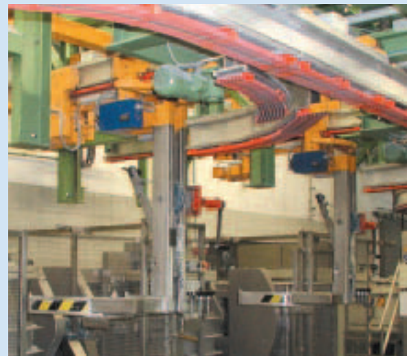
dyna-MIX with electric overhead conveying system at VARTA for the fabrication of batteries
